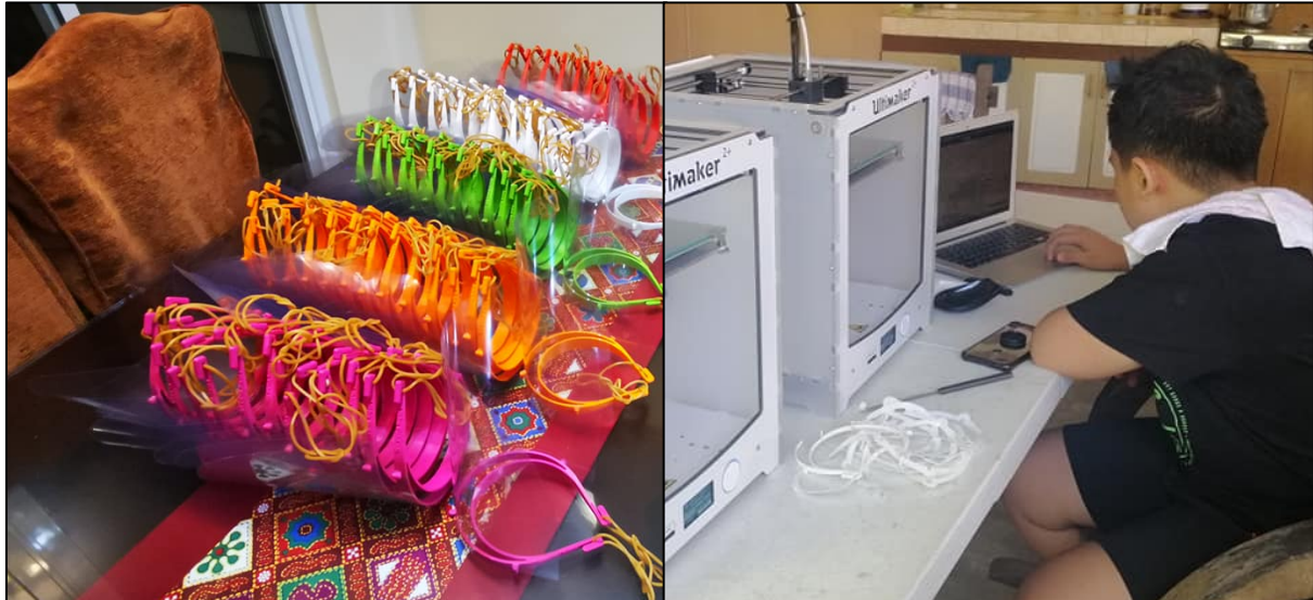
Engineers and members of the university-based LIKHA FabLab in Batangas City use 3D printing machines to create protective face masks out of acetate, rubber bands, and filament, which the team distributes to key medical facilities across the city.
