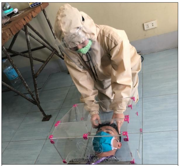
The FabLab Siquijor team tests out a protective suit made from polypropylene cloth, Velcro straps, and garter, improvised face mask and face shield made from cotton fabric, garter, filter paper, and iodized salt, and sheets of acrylic and pvc, respectively, and aerosol box used during the intubation procedure, made from acrylic sheets, 3D-printed PLA filament, and rivets.
